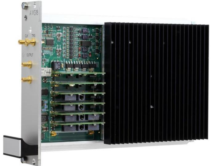
The AWG18 is an 18 bit Arbitrary Waveform Generator for high-speed / high resolution waveform generation. This module features two dedicated signal paths. A DC to 100MHz path which is optimized for accurate time domain and frequency domain measurements up to 30MHz. And a dedicated AC path optimized for signals between 10MHz to 100MHz. In combination with the built-in filters it features a typical harmonics level of better than -80dBc for the whole range.
