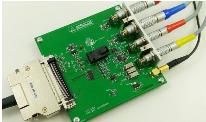
Test fixture with 4 analog signal connections
