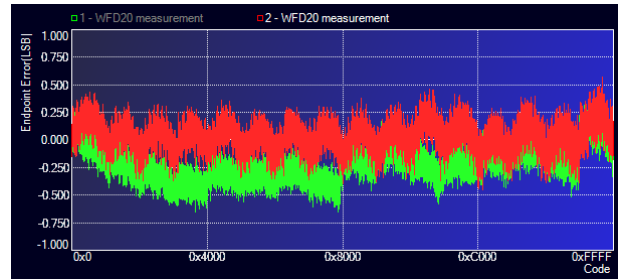
Stacked linearity result of two different 16-bit DAC devices
