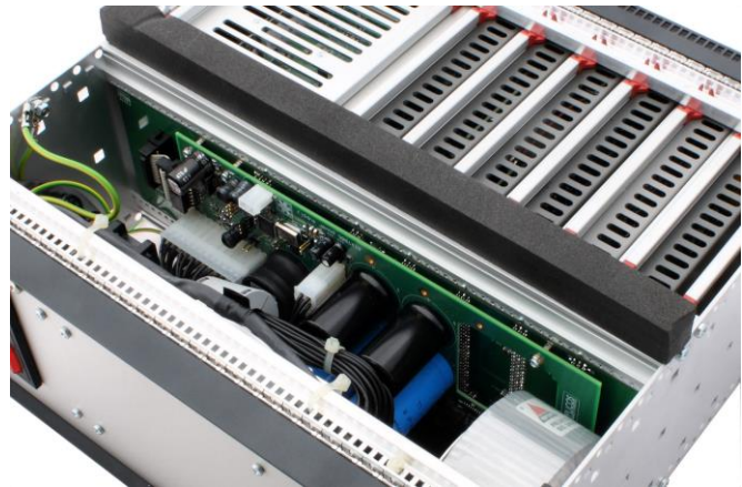
ATX-Express inside, screened modules, linear power supplies.
