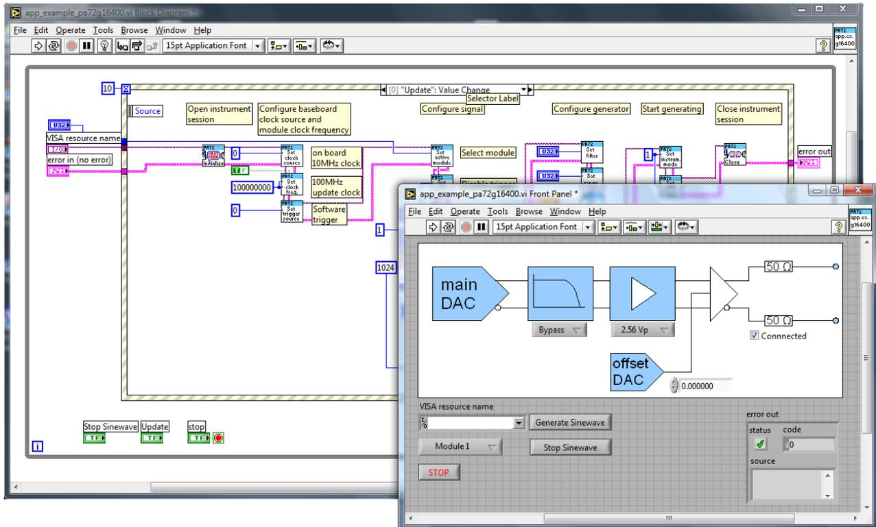
Figure 3 LabVIEW soft front panel and underlying block diagram
