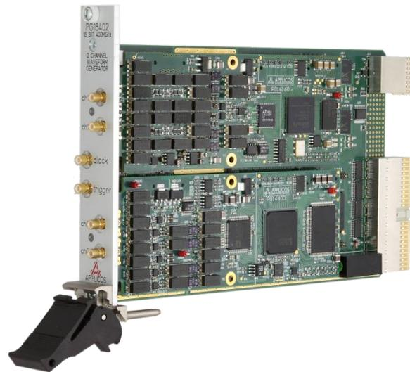
Figure 1 An example of a PXI instrument
