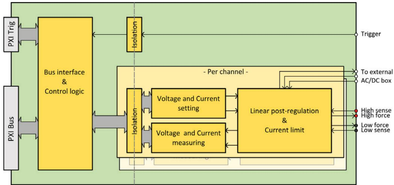
Linear regulators are used to regulate the supply voltage down to the final value. The external power box outputs a voltage just a few volts above the output voltage, controlled by the PS48402 module. This minimizes power dissipation and generated heat. The linear post-regulation used in the PS48402 ensure output noise levels in an order of magnitude lower than competitor DC/DC-conversion based output stages.
