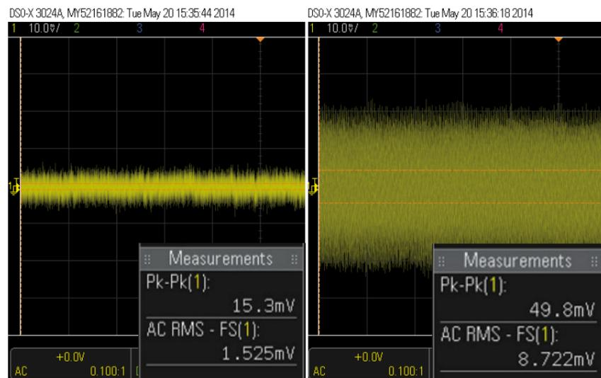
PS48402 output noise (20Hz-1MHz BW, 24V, 82Ω load)
