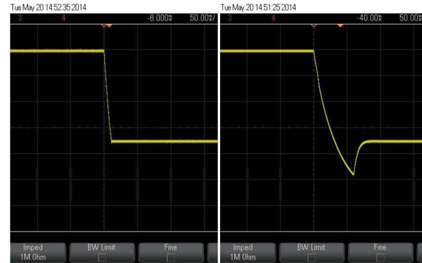
PS48402 step response (12V-5V step progr., 82Ω load)
